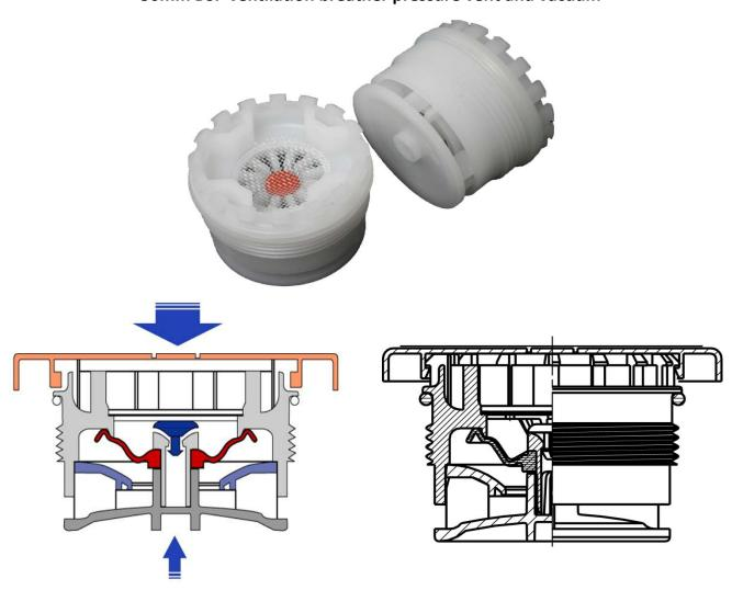
If a vacuum forms inside the inner bottle through emptying, the NBR-membrane opens and allows air to enter. If case of overpressure, the vent will open to discharge air.
